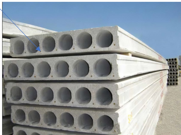
Photograph 2: Hollow-Core Plank {Example Photo}
